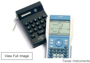
TI's first handheld electronic calculator from 1967 (left) and its latest model, the TI-Nspire, which has computer-like features.
